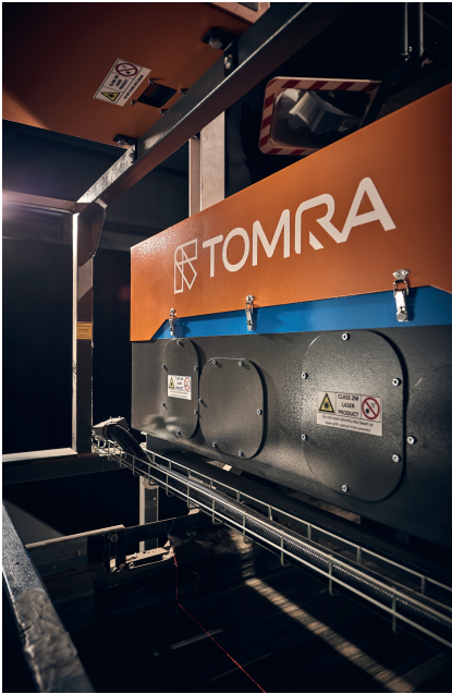
Fig. 4. Deep learning in operation: for its Auto-sort sorting machines, Tomra offers the neural network Gain, which makes it possible to sort silicone cartridges, for example © Tomra
