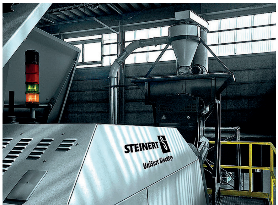
Fig. 3. The UniSort Blackeye sorting system from Steinert can also sort black plastics waste colored with carbon black © Steinert
